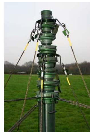
Telescopic Pneumatic Mast Supporting Racal Log Periodic Antennas
