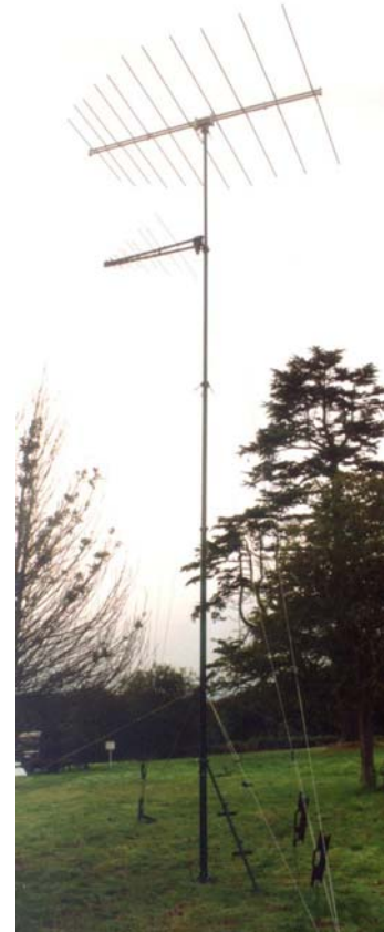
Telescopic Pneumatic Mast Supporting Racal Log Periodic Antennas
